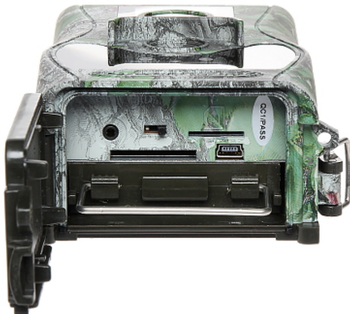
Bottom view (SD card slot, SIM card slot, mini USB, AV sockets and place for batteries):
