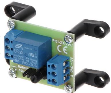
The PK1-12-ZPC allows the extension of the short trigger pulse for the time set by potentiometer.
