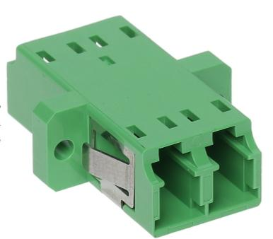
Single-mode adapter AD-2LC-APC/2LC-APC for connecting two pairs pf LC APC type plugs.
