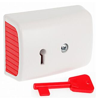
This button is a device designed to instantly trigger the alarm and (or) initiate the procedure of reporting an emergency situation in protected facility to the monitoring station. With the spring removed, the button after being pushed in will remain inside the casing (so-called, mechanical memory of use), until it is released with the key.
