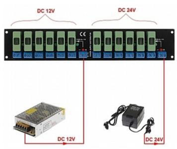
The LZ-12/R device is designed to mount in the A19-FRAME panel or as the separate device:
