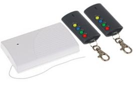
The design is based on the components of Microchip Technology Inc. KEELOQ®. It ensures both security of use and resistance to spurious control signals coming from other devices.
