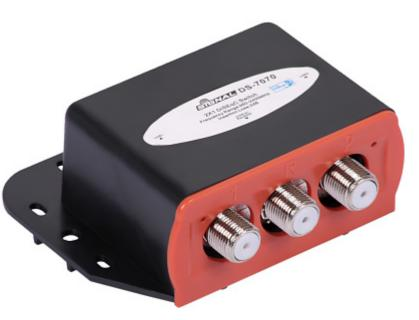
Switch allows to receive by satellite receiver the channels from 2 satellite positions (e.g. Astra and Hot Bird). The switch is controlled via DiSEqC signal in version 2.0. Switch operates with most of currently manufactured digital satellite receivers equipped with DiSEqC generator.
