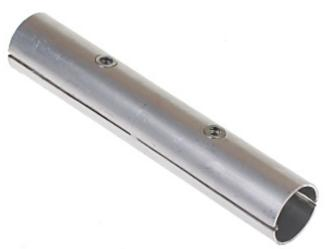
Aluminum expansion coupler for M-3.0 DURAL masts. It can be dismounted many times and using again. To connect two M-3.0 DURAL masts using coupler, you should drill the holes in each mast at a distance of 40 mm from the edge. The holes should be made in order to access to the coupler's hex screws (allen 3 mm).
