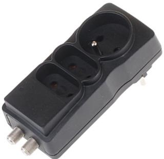
The AXON-MINI/SAT overvoltage limiter ensures continuous protection against overvoltages of three devices and TV-SAT antenna signal line. It is equipped with one grounded power outlet, two flat non-grounded power outlets and two TV-SAT phone sockets. It is perfect solution to increase the functionality of the single surface power outlet and protect TV-SAT receiver against overvoltages of SAT antenna signal line.
