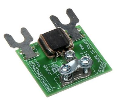
The SA/I-III-DIPOL antenna impedance transformer matches the antenna impedance to the impedance of coaxial cable.
