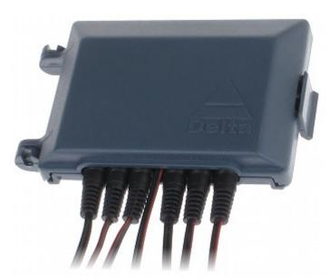
The housing construction enables easy mounting the device on a wall or mast, using tie for example:
