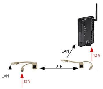
The range depends on the resistance of twisted-pair cable, current consumption of the device and an acceptable voltage drop between the power adapter and the device.
