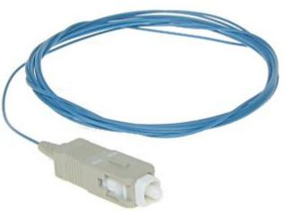
Pigtail is a short section of fiber-optic cable in the coating, one side factory terminated connector, on the other side exposed fiber. Pigtails can be stripped and fusion spliced to fibers of the distribution cable, thus avoiding the process of connectors terminating.
