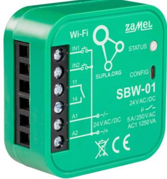
The SBW-01 controller enables remote opening and closing of swing gates, sliding gates, garage gates and doors. The device is enough to be attached to the gate operator or electric lock to be able to safely control gates and doors. Control is possible via a physical switch, a web browser, or the SUPLA mobile application.
