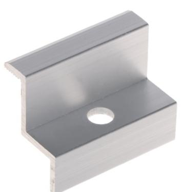
End clamp, designed for fixing extremely spaced solar panels on the mounting profile. The surface pressing the panel frame is grooved, which guarantees better grip of the panel.
