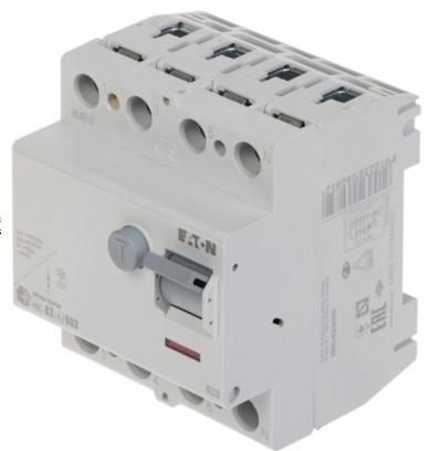
Residual current circuit breaker with rated sensitivity of I $\Delta n=30\,mA$ , AC type. The HNC-63/4/003 circuit breaker is compatible to DIN TS-35 rail mounting system.
