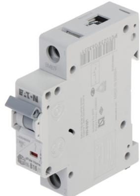
Thermal-magnetic circuit breaker with B-type curve and 16A rated current. The HN-B16/1 circuit breaker is compatible to DIN TS-35 rail mounting system.
