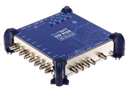
The MultiBAS devices from TELKOM-TELMOR are a combination of an amplifier and a multiswitch.
