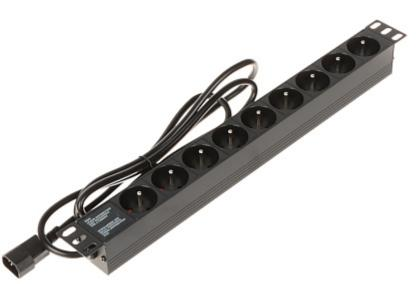
Rated voltage: 230 V AC / 50 Hz Total maximal current: 16 A Maximal total load: 3680 W 9 x CEE 7/5 Number of outlets: In RACK 19" cabinets Assembly: Length of the power cable:  $1.8\ m$  - cable with power connector IEC320 C14 1 U RACK 19" Housing type: Switch: \_ Weight: 0.75 kg Dimensions: 483 x 45 x 44 mm Guarantee: 2 years
