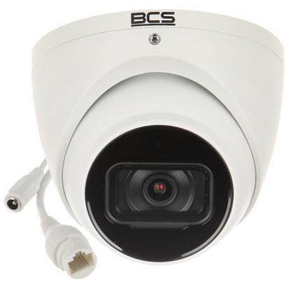
IP camera with efficient H.264 / H.265 image compression algorithm for clear and smooth video streaming at maximal resolution of 5 MPx. Due to above it is perfect solution for surveillance systems requiring persons or vehicles recognition.
