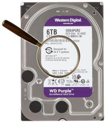
The Western Digital drives marked SURVEILLANCE HDD are designed to work in video surveillance systems. Its design allows for error-free recording of several Full HD streams in 24/7 mode. Connectors:
