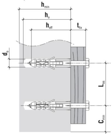
$\begin{aligned} & \text{Hole/drill diameter } [d_0] \text{ - } 14 \text{ mm} \\ & \text{Min. substrate thickness } [h_{\text{min}}] \text{ - } 120 \text{ mm} \\ & \text{Drilled hole depth } [h_0] \text{ - } 90 \text{ mm} \\ & \text{Anchorage depth } [h_{\text{eff}}] \text{ - } 80 \text{ mm} \end{aligned}$
