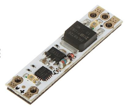
The TWILIGHT-SWITCH/BLEBOX twilight sensor is used to turn the LED lighting on and off depending on the ambient light. The "soft start" function allows to mild lightening/darkening the lighting at dusk/dawn.
