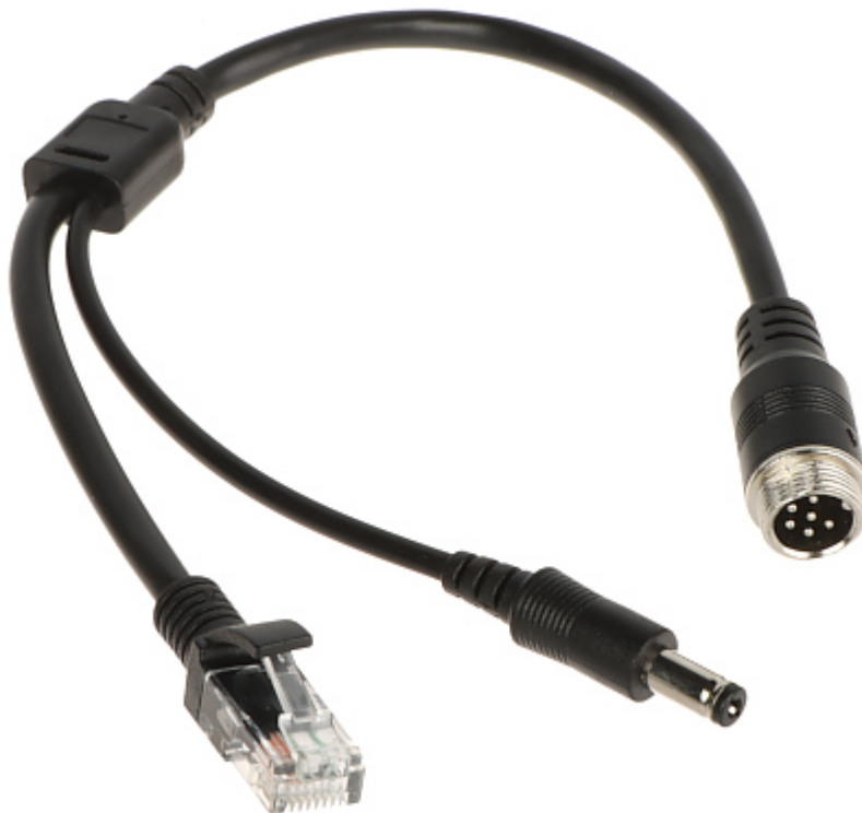
Connection cable terminated with M12 6-pin plug on one side and RJ-45 plug and 2.1/5.5mm power plug on the other.
