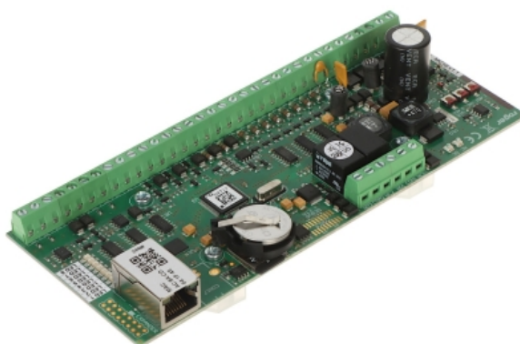
The MC16-PAC-ST-14 controller is a multifunctional electronic module, intended for use in the RACS 5 v2 system, which enables the implementation of access control of the transition and building automation.
