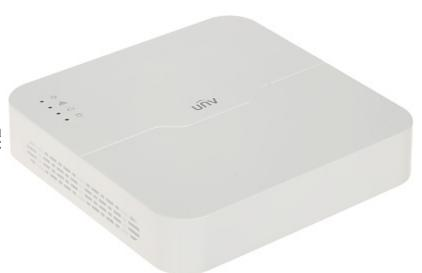
The NVR501-04B-LP4 digital recorder is a professional device using in IP surveillance systems. 4-port PoE Switch built-in.
