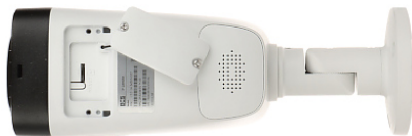
Memory card slot and "Reset" button:
