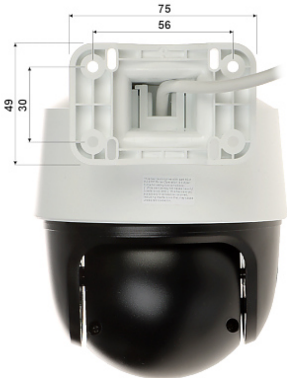
Camera mounting dimensions:
