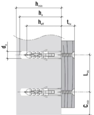
$\begin{array}{l} Hole/drill \ diameter \ [d_{o}] - 8 \ mm \\ Min. \ substrate \ thickness \ [h_{min}] - 60 \ mm \\ Drilled \ hole \ depth \ [h_{o}] - 50 \ mm \\ Anchorage \ depth \ [h_{eff}] - 40 \ mm \\ \end{array}$
