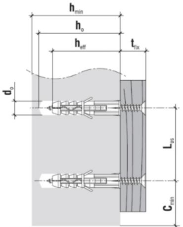
$\begin{array}{l} Hole/drill \ diameter \ [d_{o}] \ - \ 6 \ mm \\ Min. \ substrate \ thickness \ [h_{min}] \ - \ 45 \ mm \\ Drilled \ hole \ depth \ [h_{o}] \ - \ 40 \ mm \\ Anchorage \ depth \ [h_{eff}] \ - \ 30 \ mm \\ Max. \ usable \ length \ [t_{fix}] \ - \ 5 \ mm \\ \end{array}$
