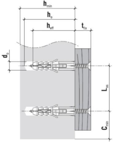
$$\begin{split} & \text{Hole/drill diameter } [d_{\text{o}}] \text{ - } 10 \text{ mm} \\ & \text{Min. substrate thickness } [h_{\text{min}}] \text{ - } 90 \text{ mm} \\ & \text{Drilled hole depth } [h_{\text{o}}] \text{ - } 70 \text{ mm} \\ & \text{Anchorage depth } [h_{\text{eff}}] \text{ - } 60 \text{ mm} \\ & \text{Max. usable length } [t_{\text{fix}}] \text{ - } 40 \text{ mm} \end{split}$$
