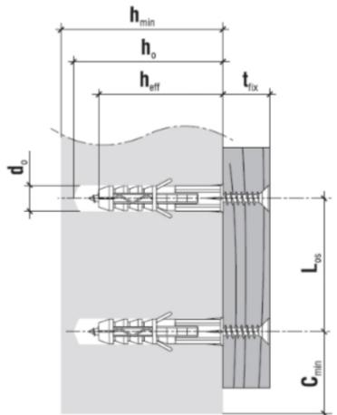
$\begin{array}{l} Hole/drill \ diameter \ [d_{o}] \ - \ 10 \ mm \\ Min. \ substrate \ thickness \ [h_{min}] \ - \ 90 \ mm \\ Drilled \ hole \ depth \ [h_{o}] \ - \ 70 \ mm \\ Anchorage \ depth \ [h_{eff}] \ - \ 60 \ mm \\ Max. \ usable \ length \ [t_{fix}] \ - \ 20 \ mm \\ Min. \ axial \ distance \ (concrete/other \ substrate) \ [L_{os}] \ - \ 120/180 \ mm \\ Min. \ distance \ from \ edge \ [c_{min}] \ - \ 120 \ mm \\ \end{array}$
