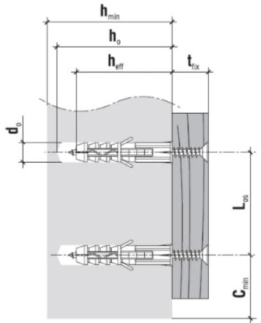
$\begin{array}{l} Hole/drill \ diameter \ [d_o] \ - \ 10 \ mm \\ Min. \ substrate \ thickness \ [h_{min}] \ - \ 90 \ mm \\ Drilled \ hole \ depth \ [h_o] \ - \ 70 \ mm \\ Anchorage \ depth \ [h_{eff}] \ - \ 60 \ mm \\ Max. \ usable \ length \ [t_{fix}] \ - \ 1 \ mm \\ Min. \ axial \ distance \ (concrete/other \ substrate) \ [L_{os}] \ - \ 120/180 \ mm \\ \end{array}$
