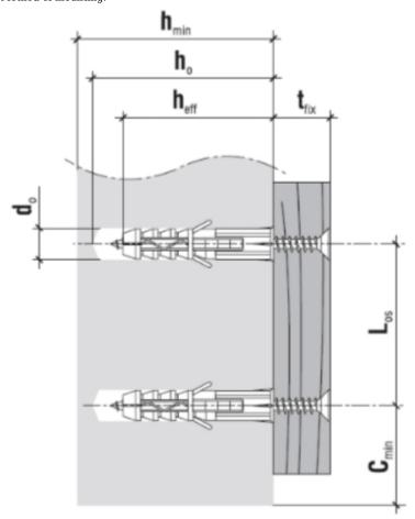
$\begin{aligned} & \text{Hole/drill diameter } [d_{\text{o}}] \text{ - } 10 \text{ mm} \\ & \text{Min. substrate thickness } [h_{\text{min}}] \text{ - } 75 \text{ mm} \\ & \text{Drilled hole depth } [h_{\text{o}}] \text{ - } 60 \text{ mm} \\ & \text{Anchorage depth } [h_{\text{eff}}] \text{ - } 50 \text{ mm} \end{aligned}$
