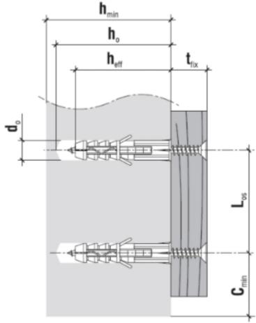
$$\begin{split} & \text{Hole/drill diameter } [d_o] \text{ - } 10 \text{ mm} \\ & \text{Min. substrate thickness } [h_{\text{min}}] \text{ - } 75 \text{ mm} \\ & \text{Drilled hole depth } [h_o] \text{ - } 60 \text{ mm} \\ & \text{Anchorage depth } [h_{\text{eff}}] \text{ - } 50 \text{ mm} \\ & \text{Max. usable length } [t_{\text{fix}}] \text{ - } 1 \text{ mm} \end{split}$$
