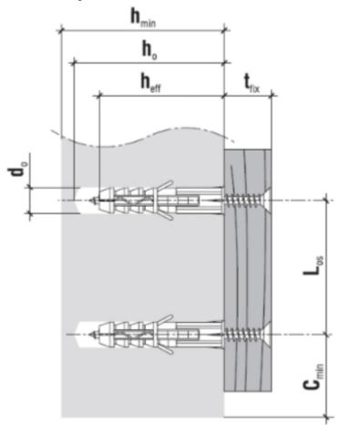
$$\begin{split} & \text{Hole/drill diameter } [d_o] \text{ - 8 mm} \\ & \text{Min. substrate thickness } [h_{\text{min}}] \text{ - 75 mm} \\ & \text{Drilled hole depth } [h_o] \text{ - 60 mm} \\ & \text{Anchorage depth } [h_{\text{eff}}] \text{ - 50 mm} \\ & \text{Max. usable length } [t_{\text{fix}}] \text{ - 30 mm} \end{split}$$
