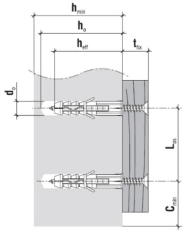
$\begin{array}{l} Hole/drill \ diameter \ [d_o] - 8 \ mm \\ Min. \ substrate \ thickness \ [h_{min}] - 60 \ mm \\ Drilled \ hole \ depth \ [h_o] - 50 \ mm \\ Anchorage \ depth \ [h_{eff}] - 40 \ mm \\ Max. \ usable \ length \ [t_{eff}] - 1 \ mm \\ Min. \ axial \ distance \ (concrete/other \ substrate) \ [L_{os}] - 80/120 \ mm \\ \end{array}$
