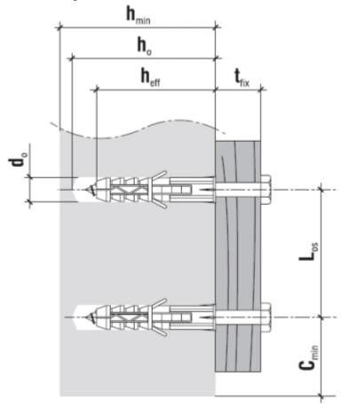
$$\label{eq:hole_drill} \begin{split} & Hole/drill\ diameter\ [d_0] - 12\ mm \\ & Min.\ substrate\ thickness\ [h_{min}] - 120\ mm \\ & Drilled\ hole\ depth\ [h_0] - 90\ mm \end{split}$$
