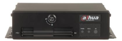
Access to the connectors on the front panel of the device is secured with a key lock:
