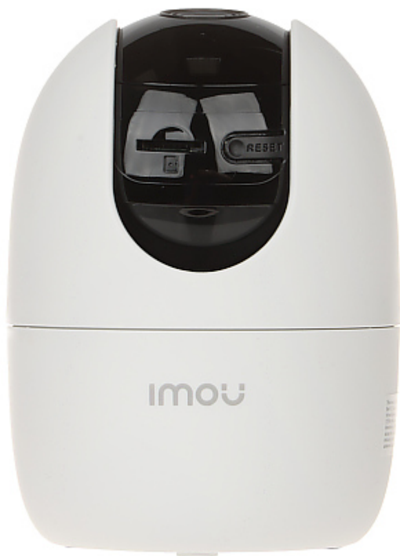
Memory card slot and "Reset" button:
