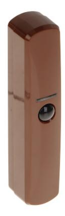
The curtain detector provides a narrow detection angle.
