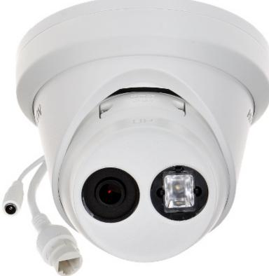
IP PTZ camera with efficient H.265 / H.264 image compression algorithm for clear and smooth video streaming at max. resolution of 1080p.
