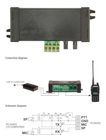
Example connection using the DIGIVOX-2 modem:
