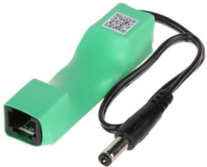
The ASDC-12-124-HS PoE adapter lowers the voltage on the DC plug to 12V and simultaneously transfers the PoE power supply to the RJ45 output. Thanks to this, from one PoE line we can simultaneously power the IP camera and additional devices powered by 12V DC.
