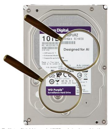
The Western Digital drives marked PURZ are designed to work in video surveillance systems. Its design allows for error-free recording of several Full HD streams in 24/7 mode. Connectors view:
