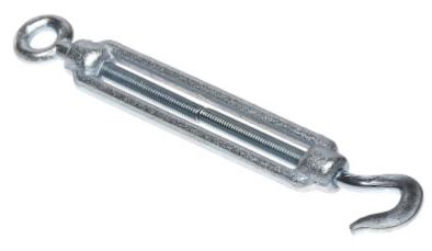
Turnbuckles are used to tightening and regulations of the lines. Tension adjustment is possible by screwing oppositely directed threads located within the body.
