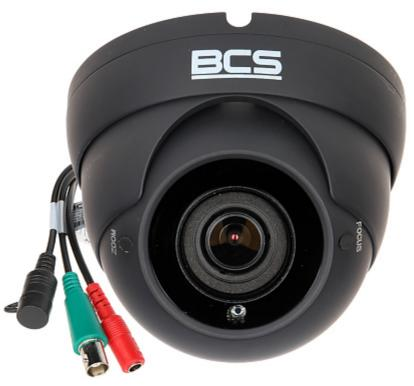
Megapixel camera with 1/2.5" CMOS sensor and AHD / HD-CVI / HD-TVI / PAL.
