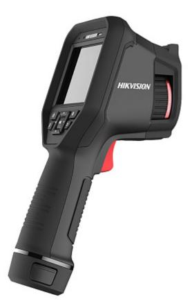
The DS-2TP21B-6AVF/W handy thermal imaging camera is equipped with a very sensitive, uncooled VOx microbolometer, allowing to obtain an image in the resolution of 160x120 px. The device will be perfect if you cannot permanently mount the thermal imaging camera and in mobile applications.
