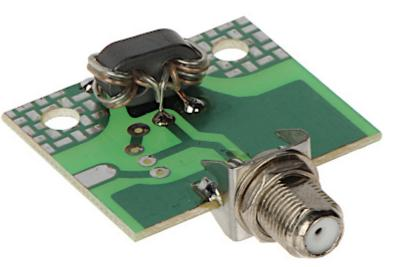
The SA/I-V/F-DIPOL antenna impedance transformer matches the antenna impedance to the impedance of coaxial cable.
