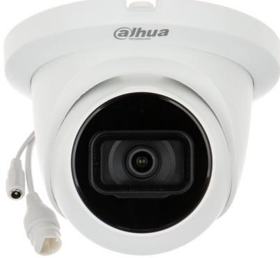
IP camera with efficient H.264 / H.265 image compression algorithm for clear and smooth video streaming at maximal resolution of 4 MPx.
